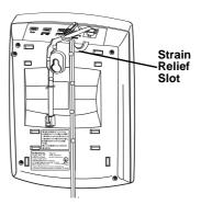
Route the end of the modular cord through the hole in the bracket, and insert the tabs on the narrow end of the bracket into the inner pair of slots near the top of the base.
